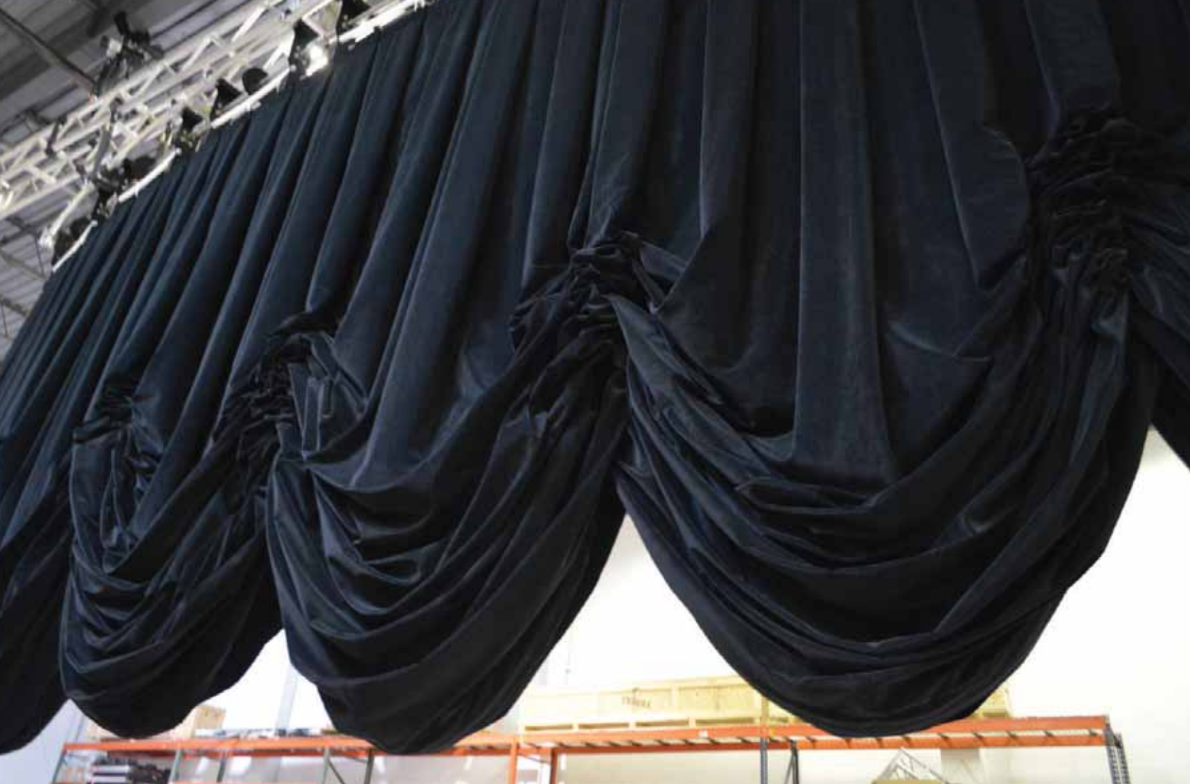
Small hoists for the individual lift lines allow the curtain to be drawn up to make one or more openings with different contours.
