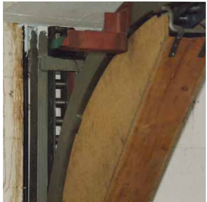
Figure 3 – Bayerische Staatsoper stage right wagon drive chain cassette
