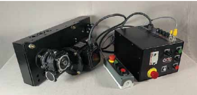
This ADC curtain machine uses a small gearmotor: powerful enough to move a curtain, but with limited power to tear things apart.
