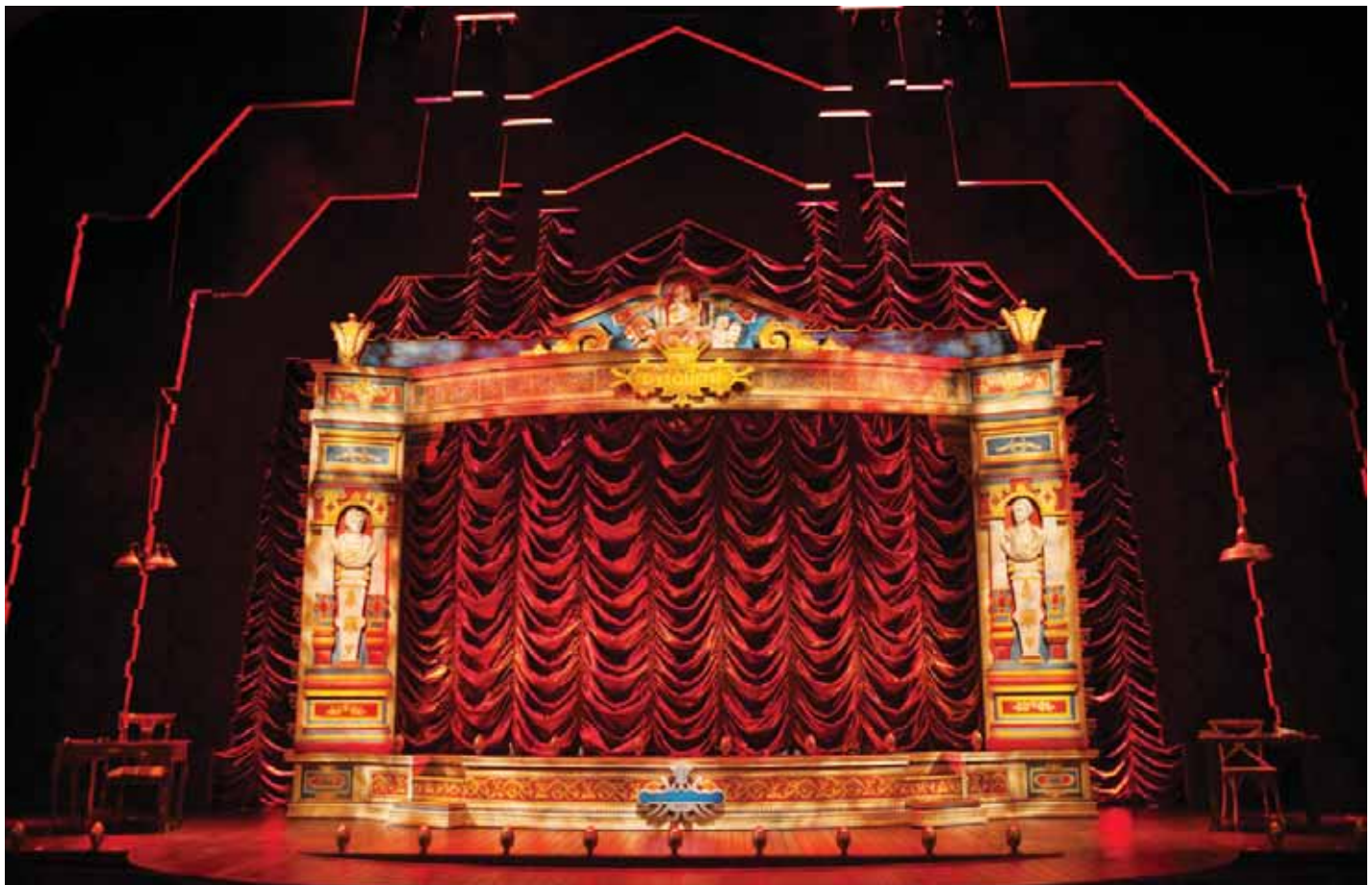
An Austrian curtain has horizontal and vertical fullness, and gathers toward the top batten as it is lifted.
